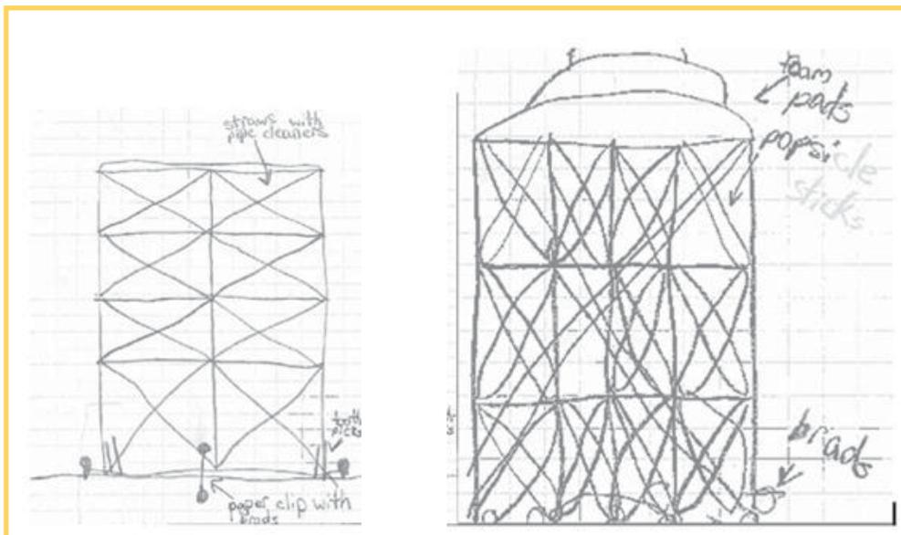
Figure 4. Plans for Earthquake-Resistant Apartment Building Model (Create step on left, Improve step on right)
